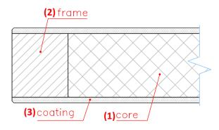
(1) The core is a chipboard based on flax fibers or wood chips with a density of 400 kg/m<sup>3</sup>.
